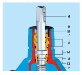
DN 250 - 400 Spindle bearing with ball bearing and additional sliding disks
