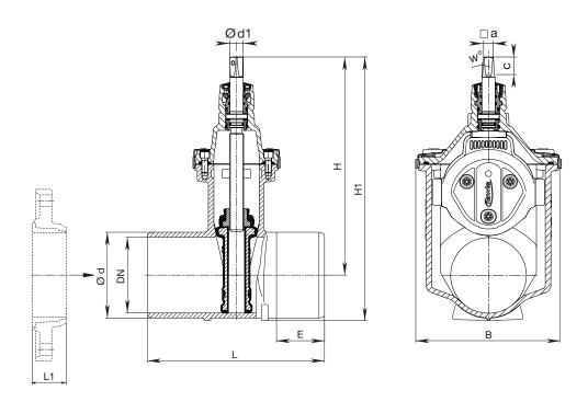
For a shorter face-to-face dimension, shorten the spigot ends<sup>1)</sup> and assemble with Hawle flanges No. 7102 / No. 0102 (see water catalogue chapter "Flange connections")
