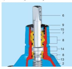
**DN 250 — 400** Spindle bearing with ball bearing and additional sliding disks
