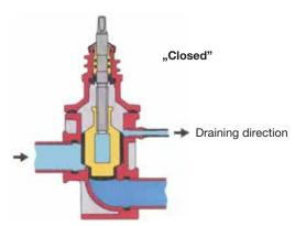
Closing torque max. 40 Nm
