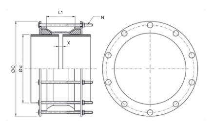
Multisize series and wide range steel fittings provide the maximum hydraulic seal, however do not restrain axial pipes movement (for this type of products please refer to the MULTIGRIP section)
