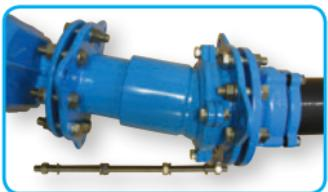
**PLEASE NOTE:** Observe the installation direction of the tension rod assembly. The dished side of all rounded washers must point inward.
