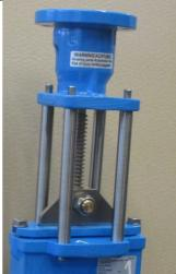
Position the adapter between the 4 tie bars by turning the spindle counter-clockwise.
