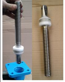
8. Exchange and grease spindle as needed.
