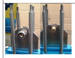
5. Remove lock nut and washer. Exchange spindle nut.
