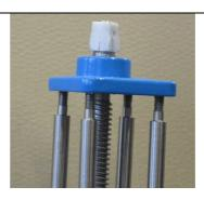
Remove bearing block by turning the spindle clockwise.
