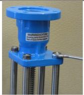
Fasten the adapter by means of washers and nuts/bolts.
