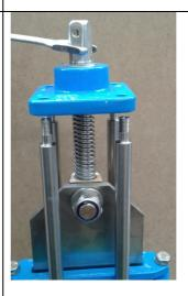
4. Remove bearing block by turning the spindle clockwise.
