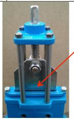
6. Grease plate with silicone grease.
