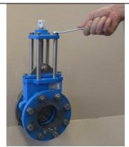
Loosen bolts between bearing block and tie bars.
