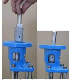
Put the spindle coupling box with the trunnion onto the spindle square in such a way that the bores coincide.
